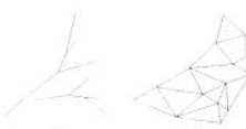
Figure 11.7. TWO NETWORK CATEGORIES: BRANCHING NETWORKS (A) WITHOUT CLOSED LOOPS AND CIRCUIT NETWORKS (WITH CLOSED LOOPS).
